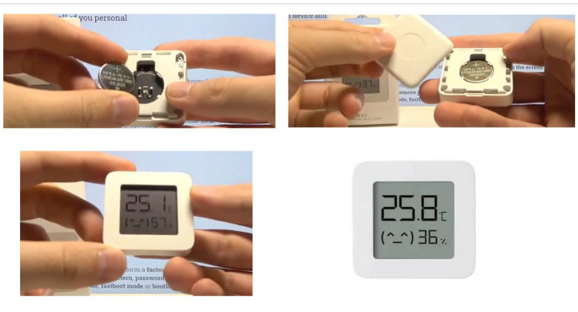
Figure 35: Battery placement into the temperature and humidity sensor
