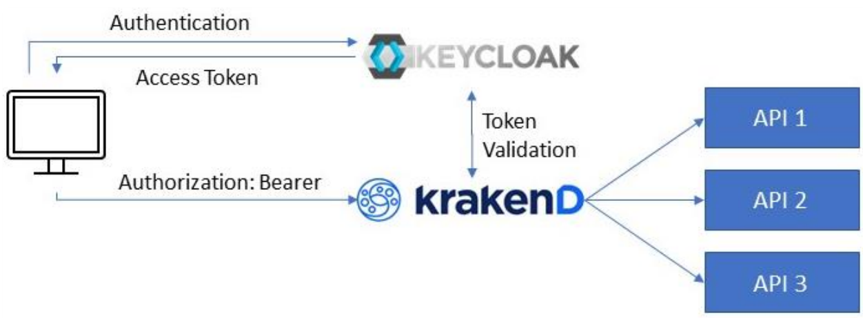
Figure 49: The Access token is been issued by Keycloak then KrakenD allows the triggering of an endpoint if role policy permits.
